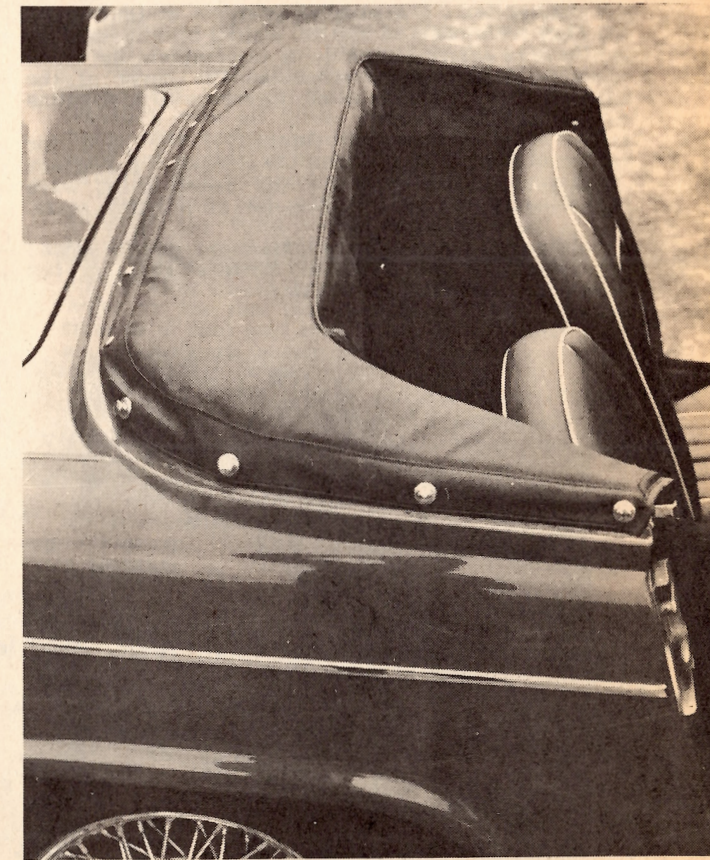
Hood stores behind seats under smooth-fitting half-tonneau, a great improvement on old system.
