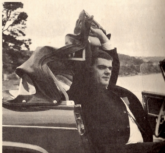
Best feature of the new car is the quick-fold hood. It can be pushed down or up one-handed.
