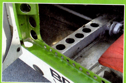
ABOVE: Holes were cut into every possible place to reduce weight.
