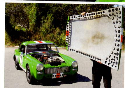
RIGHT: Neville Mansfield shows off the lightweight aluminium bonnet - one of a number of alloy panels shipped from the UK especially for the car.
