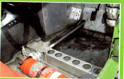
ABOVE: Driver's-side footwell, showing how the floor was lowered. Note the front suspension torsion bar.
