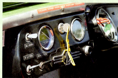
ABOVE AND LEFT: Frank van der Worm fitted a modified Midget dash to make the car look more like a Midget inside. Note the Dymo label on the top dash rail, which is copied from the original used in the 1967 Surfers 12-Hour race and says: Please sound horn when passing Ferrari.
